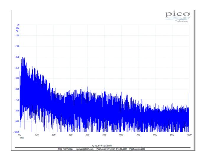
h. Here is the test of the frequencies now present with a Sine Tamer installed. You will note the large amplitudes of the frequencies previously present are reduced dramatically. This is because the Sine Tamer is rated to mitigate from 1 kHz to 10 MHz in frequency. The ground switch was on. These are dramatic results. GS unit were at 45.
