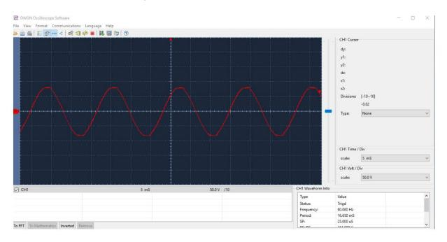
d. This is a test of the ground to neutral connection. I found no unusual effects here. The yellow trace does not show any transients or harmonics This waveform is normal.
