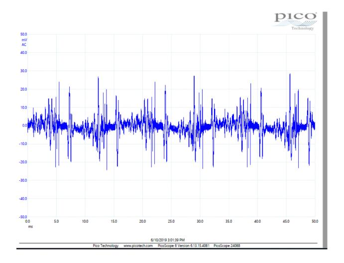
g. Now let's look at the frequencies present in the wave form. This test is for frequencies from 60 Hz to 100 kHz. You will notice that the bulk of strong signals are less than 60 kHz. What this mean is that much of what your home is experiencing is from a combination of the grid and the electric meter artifacts. This test was done with the ground circuit on. You have no electronic devices in your home that are the likely source of these frequencies.
