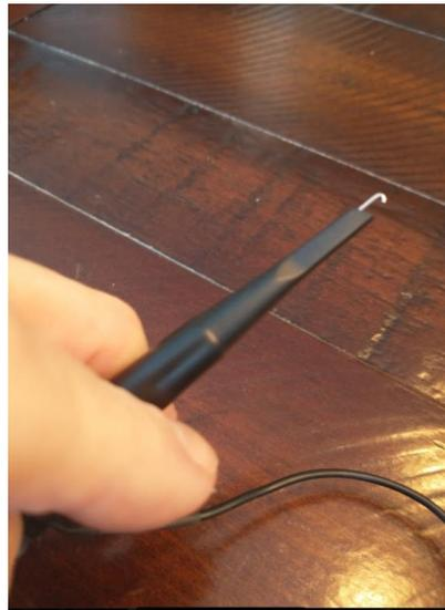
Use Spectrum View –Take the tip probe and connect it to the white wire and take the alligator clip and connect it to the green (Ground) wire. Connect the probe to the B Channel. You can try flipping this around using the probe tip and hooking it to ground and the clip to neutral. Set the probe to X1 not X10. It is safe to touch these wires because there is no power present. You cannot do a test like this with any plug in meter.
